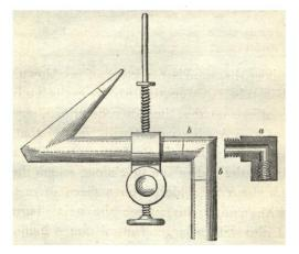
By having an elbow-joint, a section of which is seen at a in the annexed figure, and screwed in its place at b b,
